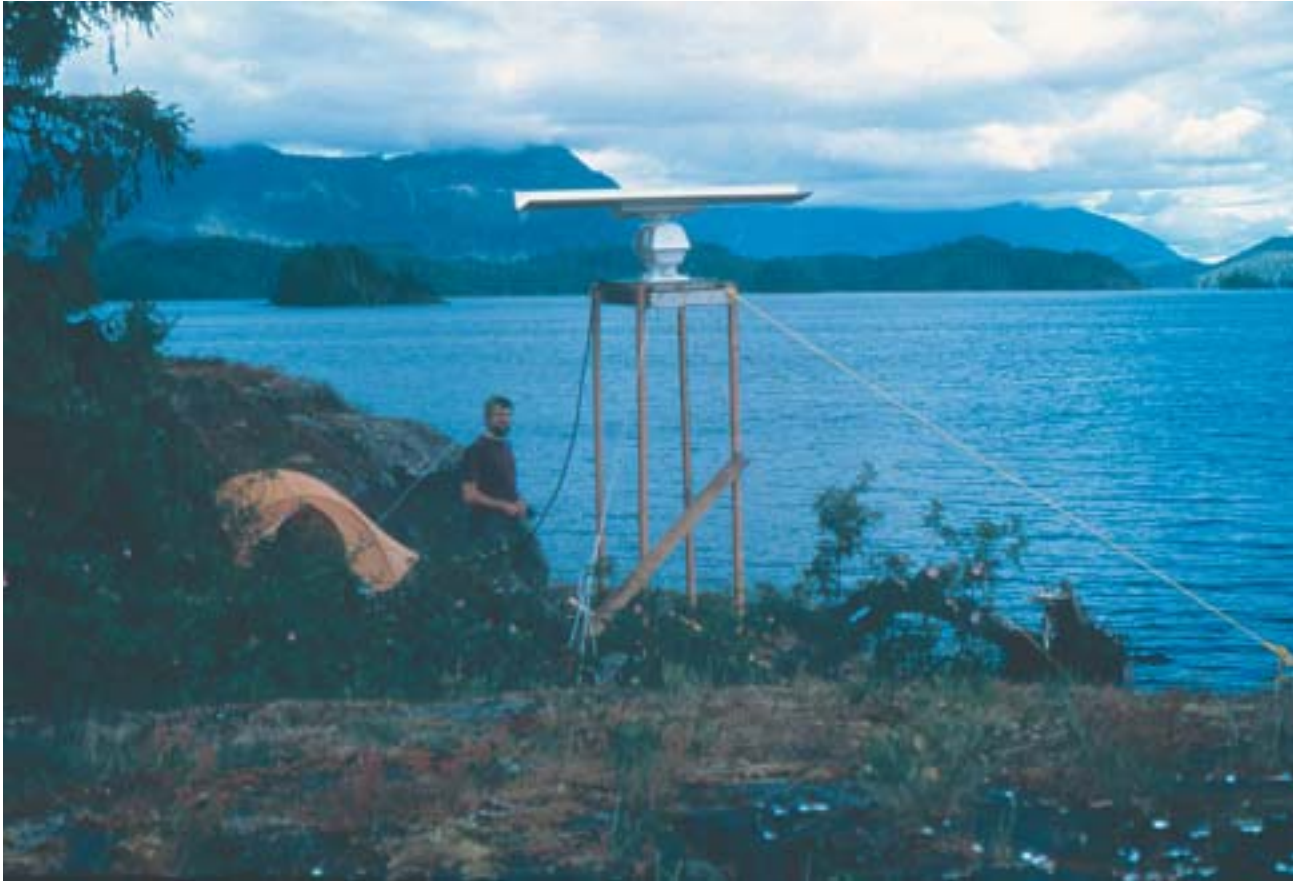
Radar set-up at mouth of Cypre Creek. High frequency scanning radar was used to count incoming birds at 19 stations in Clayoquot Sound. (photo by Andrea Lawrence)
